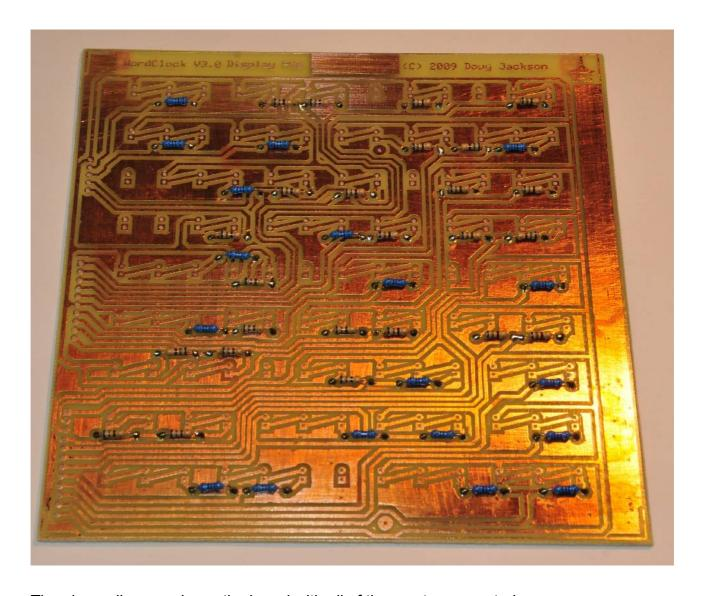
The above diagram shows the board with all of the resstors mounted.
