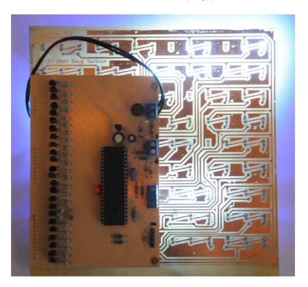
The following picture shows a closeup of the pin layout on the display PCB when it is used with a Microchip PIC controller PCB.
