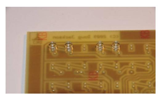
The first four LEDS installed.
