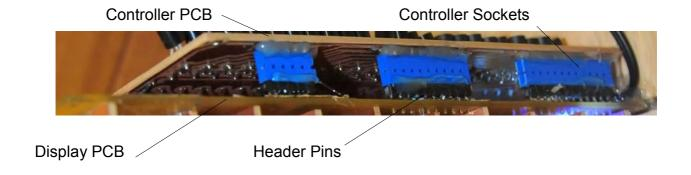
If you are constructing an Arduino based clock, you need to solder the 26 way ribon cable onto the appropriate pads on the display board. Simply strip and tin the cable into the 26 individual wires, and solder the relevant wire into the display pad, as per the following diagrams:
