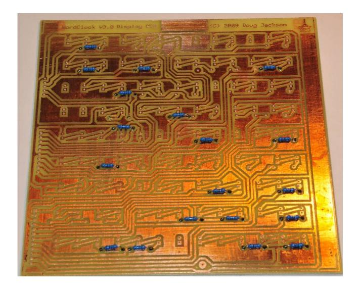
The above diagram shows the location of the 360R resistors.
