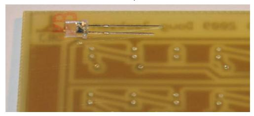
Start by inserting a group of LEDs, solder one lead, turn the board over and verify that the LED is flush against the base of the board. Move the LED closer to the board while applying heat from your soldering iron if it needs to be closer. Complete soldering by soldering in the other lead.
