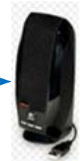
Non-powered speaker driven by PicoBoo's 10W output and amplified by an old stereo receiver
