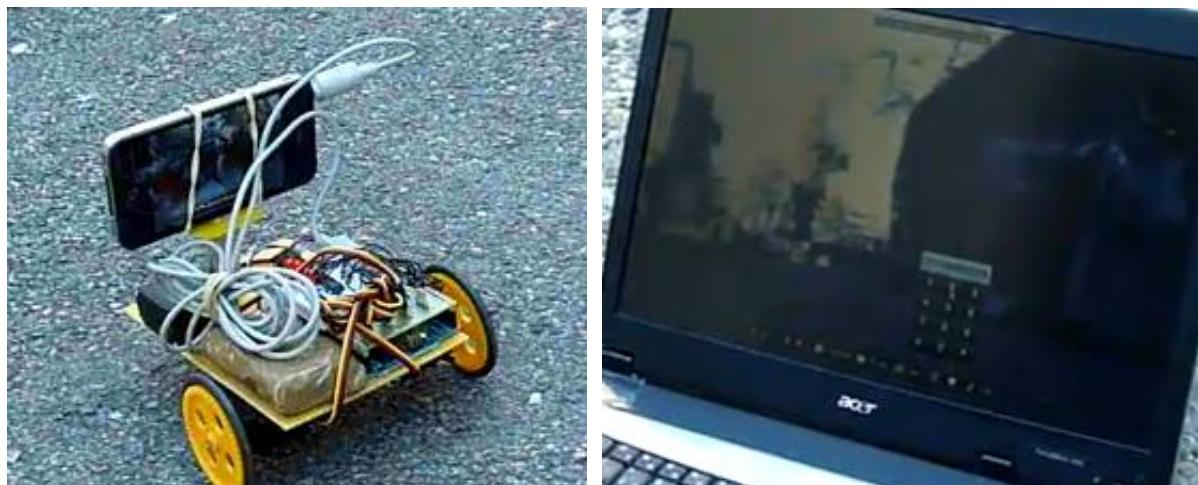
Dual frequency DTMF method is quite reliable and there exists a specialized decoder chip. DTMF chip is read out by Arduino board that controls servos.
