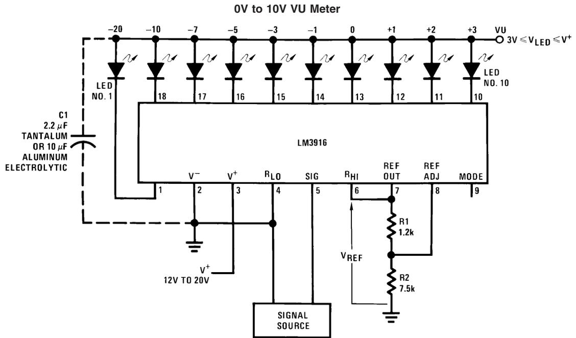
$$V_{REF} = 1.25V \left( 1 + \frac{R_2}{R_1} \right) + R_2 \times 80 \mu A$$
