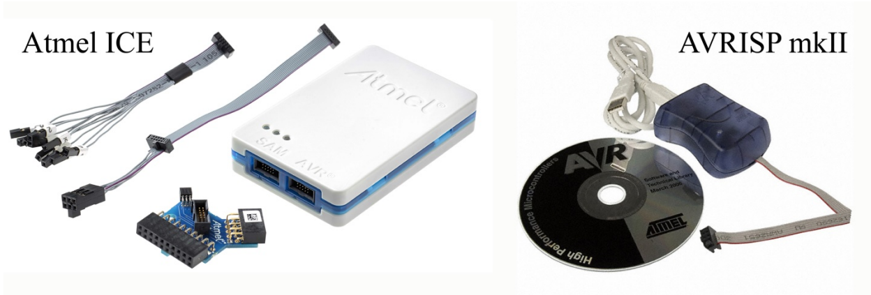
Figure 3: Atmel ICE (left) and AVRISP mkII (right) programmers. The Basic version for ICE includes the USB cable and the cable 2 nd from the top left.
