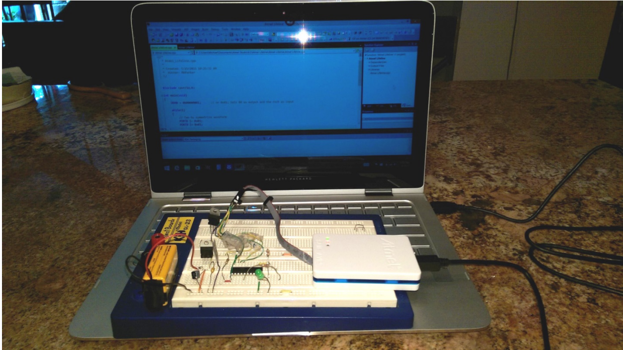
Figure 1: Laptop, programmer and experimenter's breadboard
