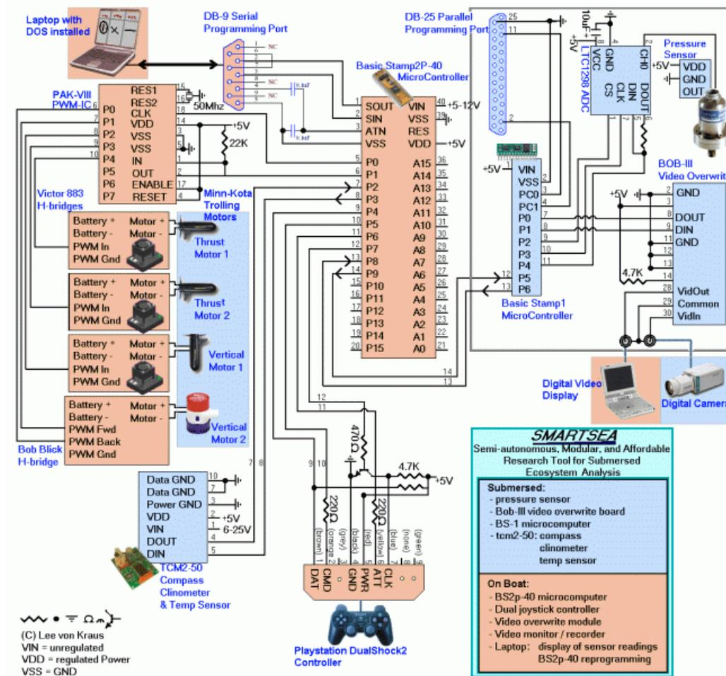
**Figure 1:** a circuit diagram showing the entire SMARTSEA electronics system. In the upper right is the video overwrite module (contains BOB-III, pressure sensor, ADC, and Basic Stamp1). In the center is the Basic Stamp 2p-40 microcontroller which serves as the middle man between the sensors, controller, laptop, and motors.
