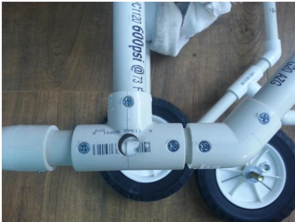
5. For the front Caster wheel, cut a short piece of PVC pipe approximately  $\frac{3}{4}$ " long. Use Duct tape to wrap around the stem of the caster till the diameter can be snugly fit inside the  $\frac{1}{2}$ " PVC pipe as shown. Then insert the caster with duct tape and PVC pipe into the front TEE piece as shown.
