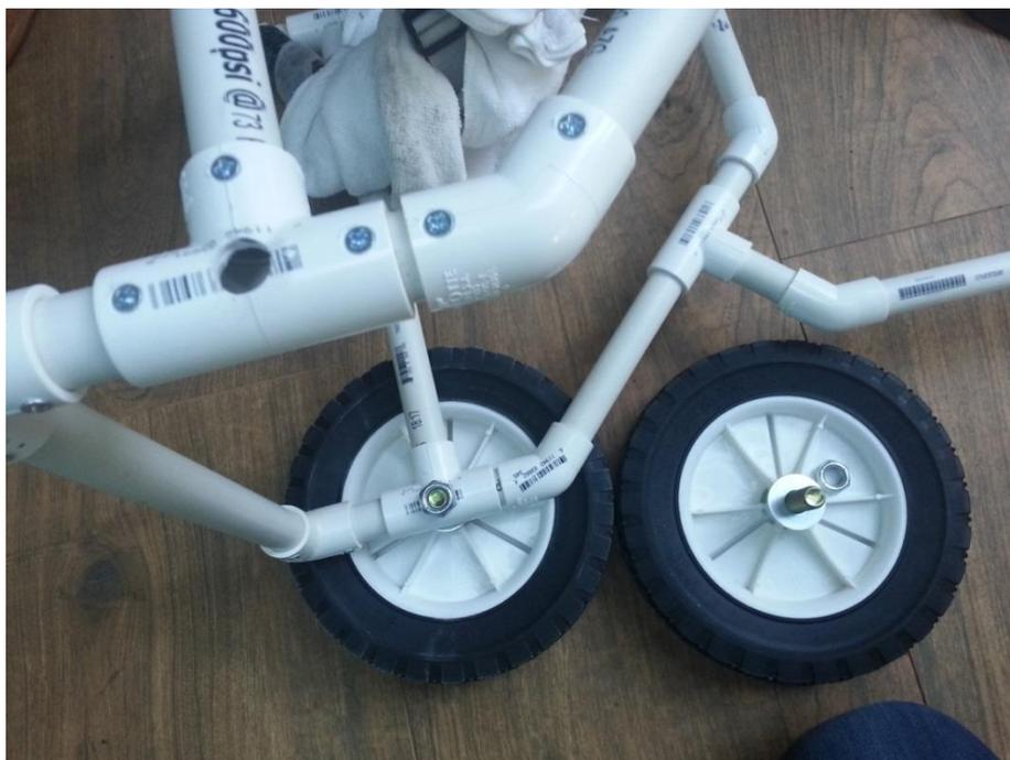
7. Body support: Note: this instruction does not include the detail of the body support. The rear body support was transferred from the old wheel chair. As shown in the picture, one can be constructed using steel rod, plastic hook, foam tube, ... items that can be acquired from general hardware store. For the front body, luggage strap was used. soft fabric can be added for more comfort. Pictures shown as examples:
