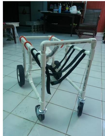
8. Size adjustment: with Messi strap into the wheel chair, I have to reduce the length by about 2.5" so that the front wheel casters will approximately line up with his front legs.
