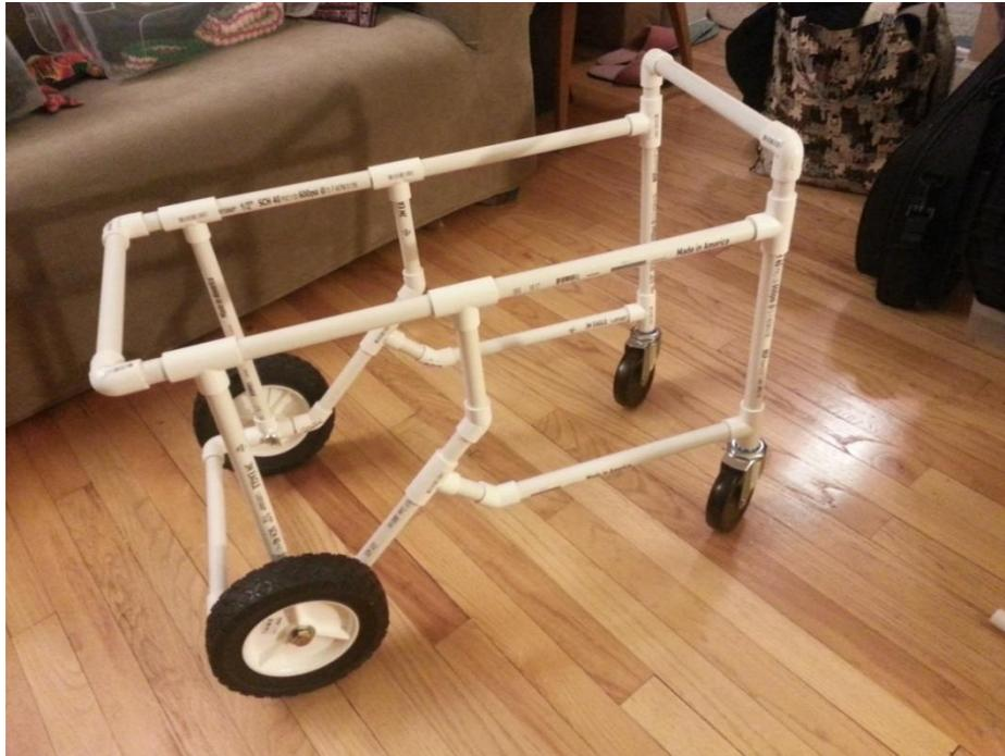
4. For this prototype, I use #6 wood screws to hold all the joint together as shown. Only one screw per joint. Use the #6 drill with countersink at approximately  $\frac{1}{2}$ " from the edge of each joint piece.
