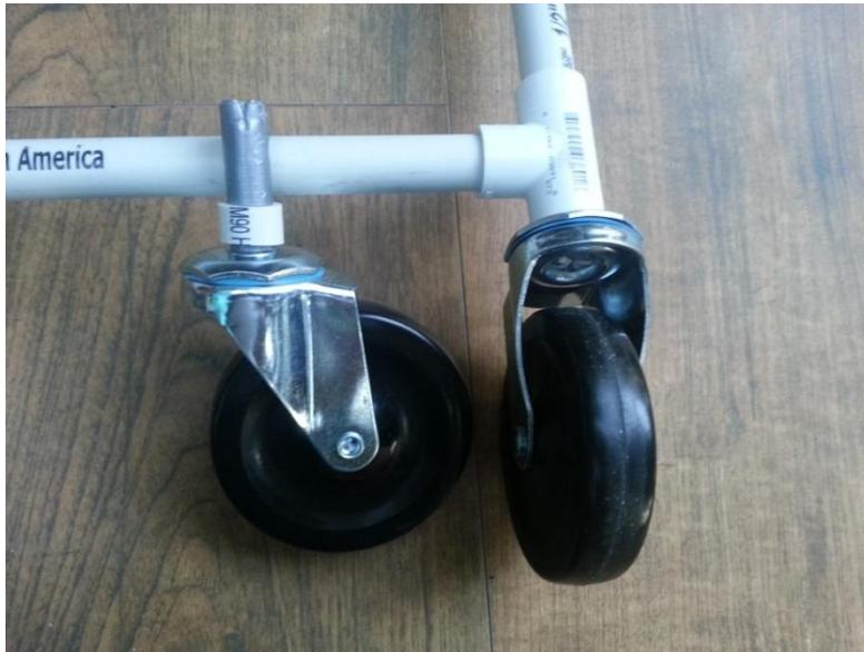
6. Assemble the Rear wheel into the  $\frac{1}{2}$ " hole of the TEE piece using the axle bolt, washer and locknut as shown.
