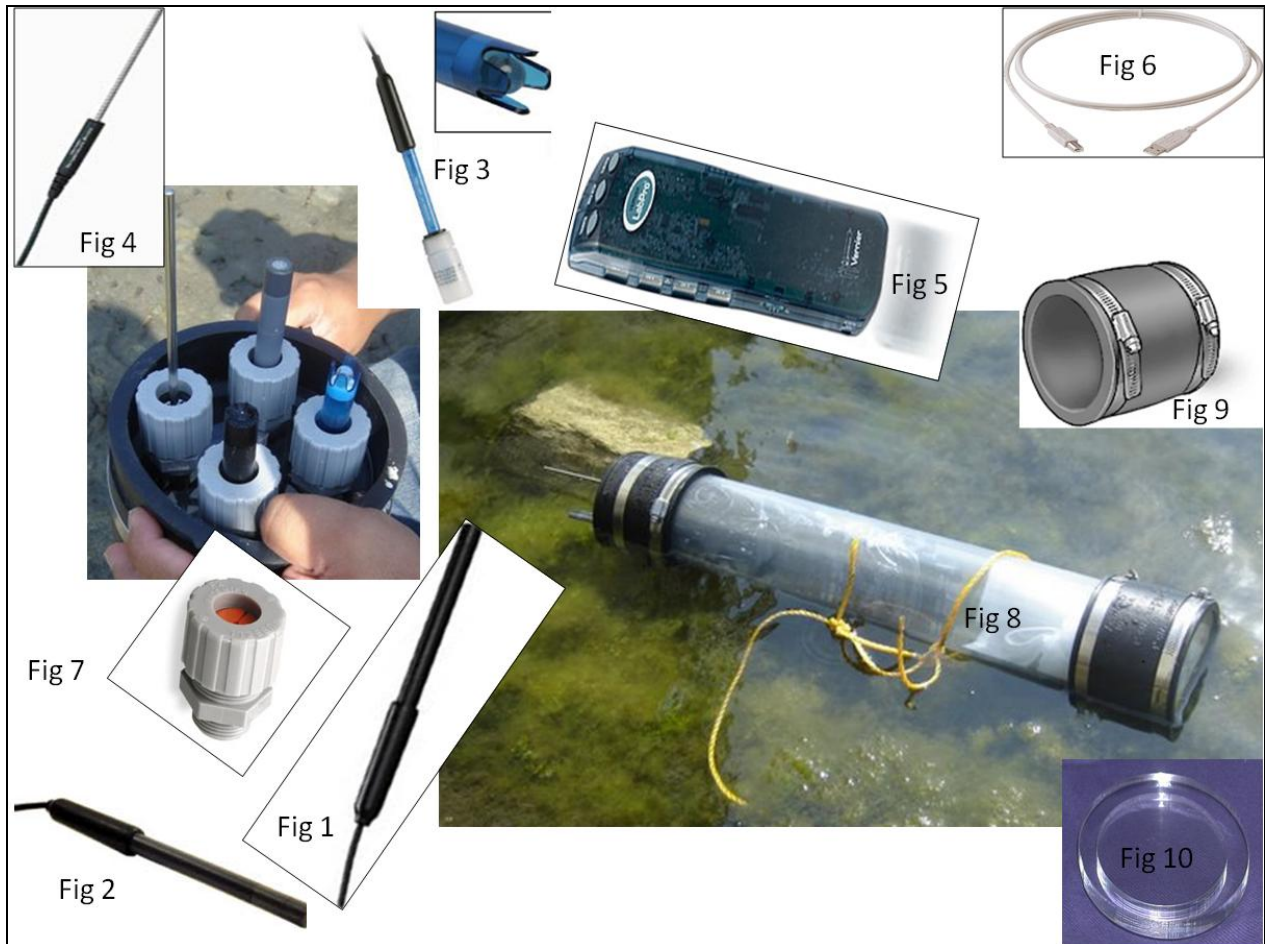
Figure 2. Overview of the components (Figures 1 to 10) used to integrate the EcoSub.
