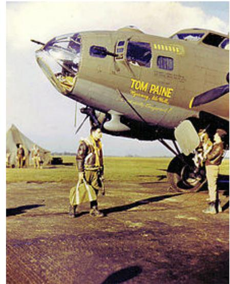
The RDF antenna on this B-17F is located in the prominent teardrop housing under the nose.
