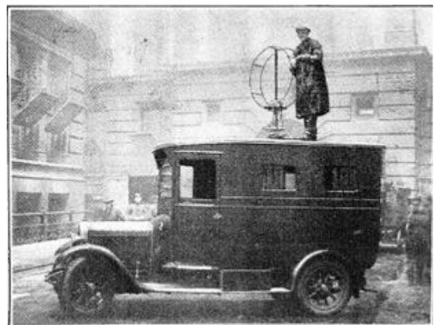
British Post Office RDF lorry from 1927 for finding unlicensed amateur radio transmitters. It was also used to find regenerative receivers which radiated interfering signals due to feedback, a big problem at the time.
