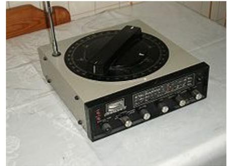
A portable, battery operated GT-302 Accumatic automatic direction finder for marine use
