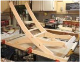
6 - Do the same in the low position. If cut and assembled correctly, the dowel should line up square and solid in the grooves in Parts B.
