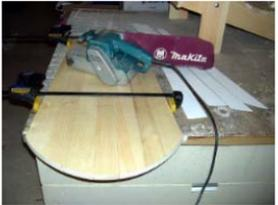
3 - For all tapered back slats, cut to the rough dimensions of part G, the longest slat. Then trace on template G, and taper the one side for all parts G, H, I & J. The templates for H, I & J can be traced onto the tapered stock, so all parts are the same width at the bottom. Only one template of each is necessary. Just flip each over for the opposite direction of the curve. When you have cut & planed or sanded all slats, assemble & clamp as shown, so you can sand the curve smooth and even.
