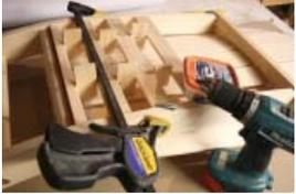
16 - If you are adding the magazine rack Parts M, trim to fit snugly between Parts A, 1/16" (1.5mm) set in, and 1 1/2" (3.8cm) apart as shown. Drill pilot holes for the brads, and glue and tack in place. Fill the holes and sand smooth..
