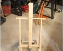
9 - Mark the center point on Parts C & D, align Part G the center back slat with the marks, and screw in position being sure it does not extend past the first dowel E. The template holes should align correctly.
