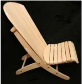
The chair is now assembled, and ready for finishing. If you are painting the chair, it is best to prime all surfaces first before assembly, to ensure longer life against moisture. Use an oil based paint like Varathane Colors, for the final coat. You can either countersink and plug the screw holes before final painting, or use brass screws left exposed if staining.
