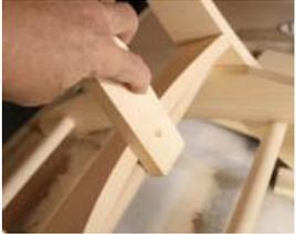
8 - Trim Part D, the lower back support, so it fits flush between parts A, resting on the top Part E dowel. Use back slat Part G to be sure Part D is on the same plane as the top back support C. Drill pilot holes on each side of Parts A, or use your counter sink bit, if plugging the holes. Screw in place with 2 screws on each side.
