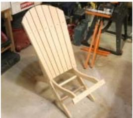
12 -After marking the center points of each slat and clamping them together to prevent movement, drill pilot holes, or use your counter sink bit if plugging the holes, and screw all slats in place into Part C & D.
