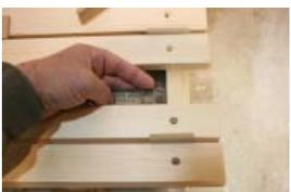
13 - After marking the center points on parts L, laid in line with the first slat, use the spacers and line up all parts.
