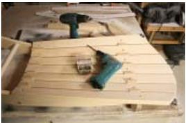
10 - Lay the back section on your assembly table, then cut up small sections of 1/4" (6mm) MDF or plywood to use as spacers for the back, as well as the seat slats. Lay all slats in position with the spacers between, aligning the top curve.
