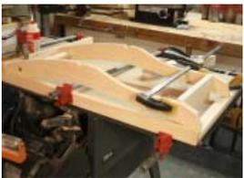
4 - Next do the same as step 3 for side panels Parts B and dowel Part F. Cut a spacer to fit at the front end and clamp to be sure the frame is square. Add a blocker to the far end, and a scrap under the front as shown....this will allow you to centre the first seat slat Parts L, flush with the front edges of Parts B. Drill pilot holes, or use your counter sink bit, if plugging the holes, and screw in place.
