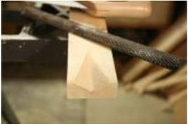
11 - All slats should align correctly, but the outer slats Parts J, will not lay flat against the edges of Parts A. Mark a notch as shown on the bottom underside of each part J, and cut out a small notch with a hand saw, until the back of the slat fits flush.
