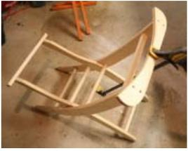
7 - Add a spacer between the tops of Parts A, being sure they are parallel, and clamp Part C centered flush with the front of Parts A. Drill pilot holes, or use your counter sink bit, if plugging the holes. Screw in place.
