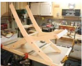
5 - You can now take the assembled back and seat and test fit together in the high position.
