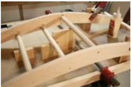
2 - Cut scraps to fit under Parts E, to ease in the glueing assembly. Apply waterproof glue to dowel ends and holes, and insert into the mating Parts A. Clamp in place being sure to check for square against your assembly table edges as well as perpendicular to the table.
