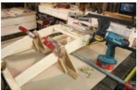
3 - It is recommended to let the glue dry completely before drilling the pilot holes for the furniture screws, since if you are drilling by hand, there may be a tendency to wander off square. If this happens and you haven't let the glue set, the side panels may go out of square after the clamps are removed....take a break, have a coffee...or whatever !
