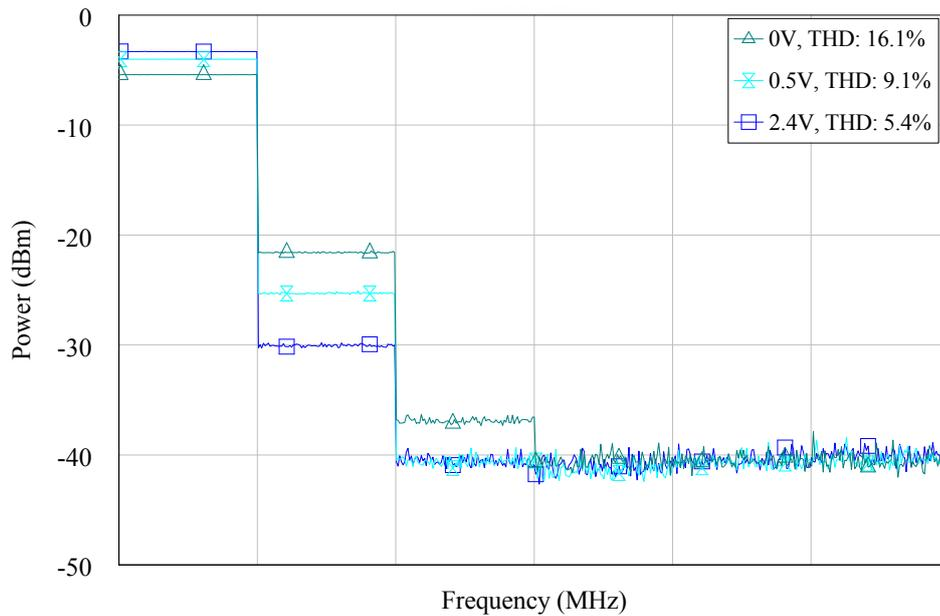
**Figure 3.16:** Fet bias influence on harmonic distortion (100MHz@20dBm)
