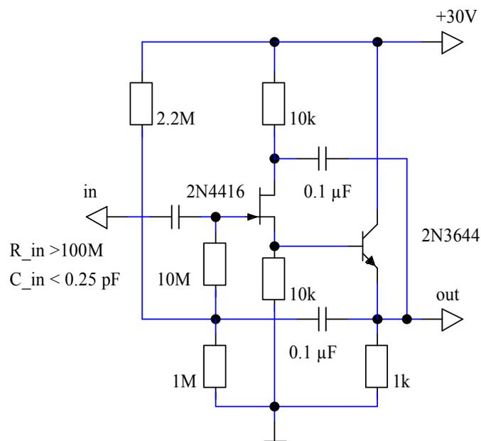
**Figure 1.2:** schematic of bootstrapped Fet
