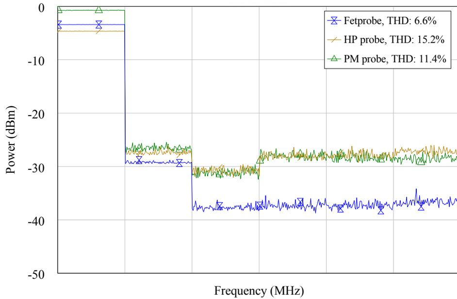
Figure 3.25: THD of Fetprobe and commercial probes (100 MHz@20 dBm)
