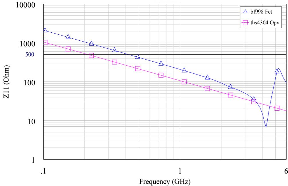
Figure 2.2: Z11 of bare devices
