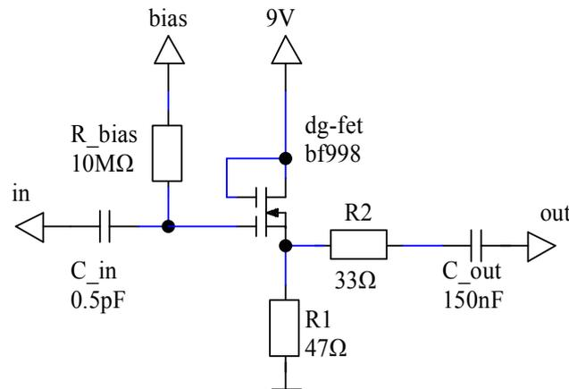
**Figure 2.3:** schematic of Fetprobe
