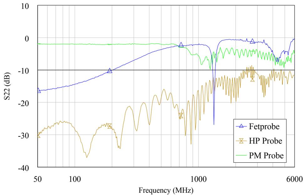
**Figure 3.19:** S22 of Fetprobe and commercial probes
