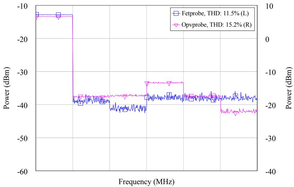
Figure 3.12: THD comparison of both active probes (10 MHz@10 dBm)
