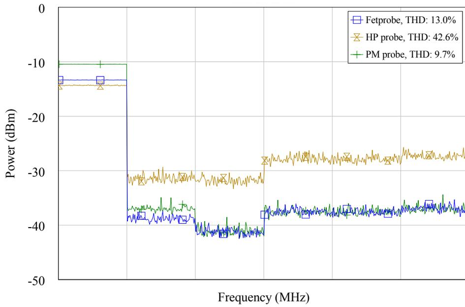
Figure 3.24: THD of Fetprobe and commercial probes (100 MHz@10 dBm)
