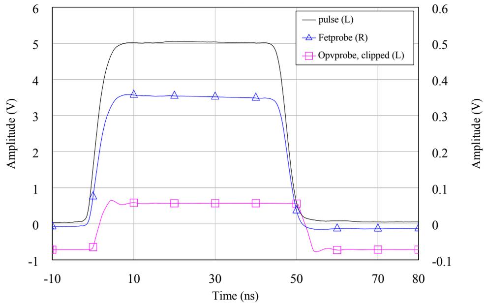
**Figure 3.10:** responses of both active probes to 5V 50ns pulse
