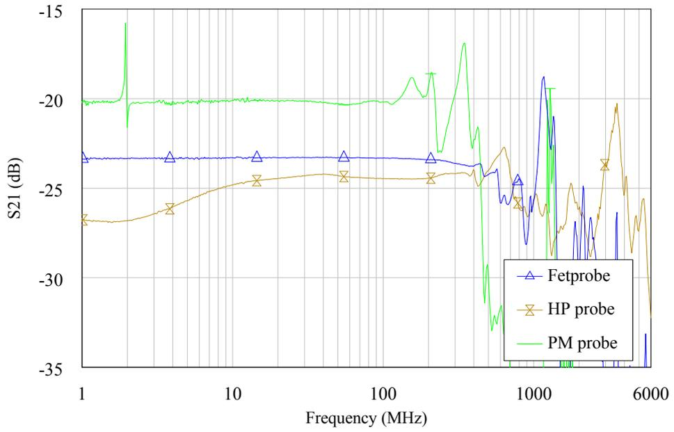
Figure 3.17:  $S_{21}$  of Fetprobe and commercial probes
