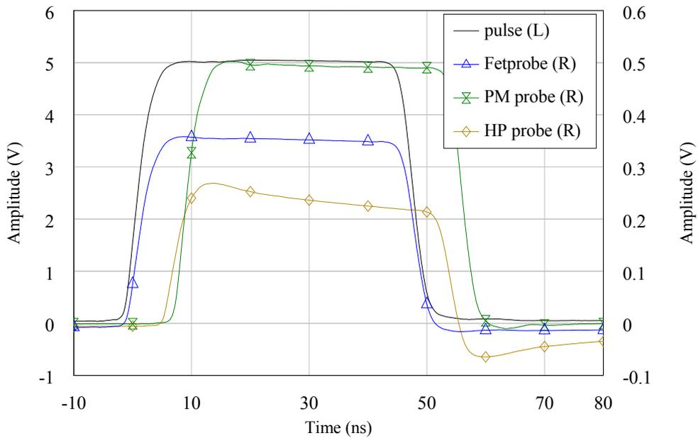
**Figure 3.21:** responses of both active probes to 5V 50ns pulse
