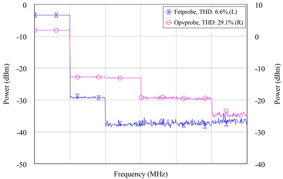
Figure 3.15: THD comparison of both active probes (100 MHz@20 dBm)
