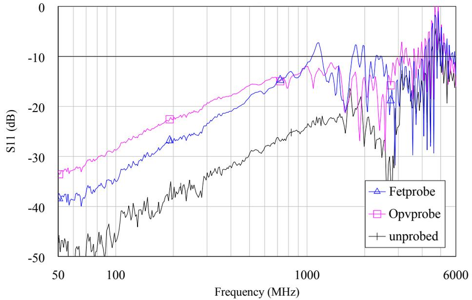
**Figure 3.6:** Input return loss of both active probes
