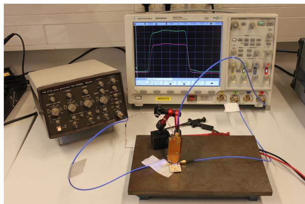
**Figure 3.8:** pulse response setup
