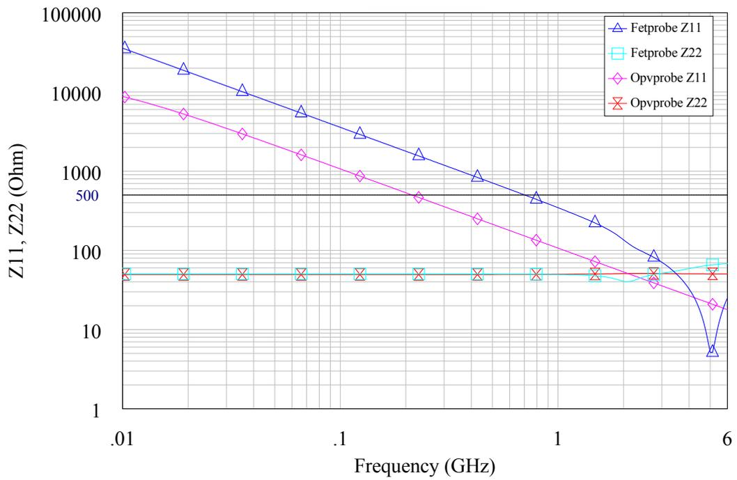
Figure 2.7: Z11 and Z22 of Fetprobe and Opvprobe
