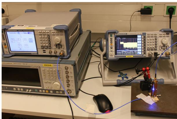
**Figure 3.11:** harmonic distortion setup
