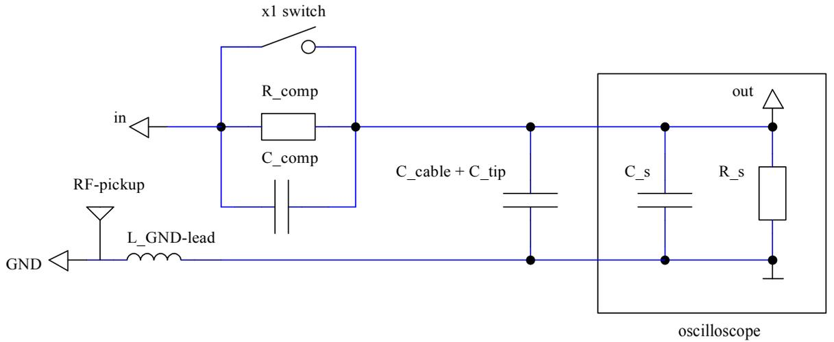
**Figure 1.1:** equivalent diagram of the oscilloscope-probe system
