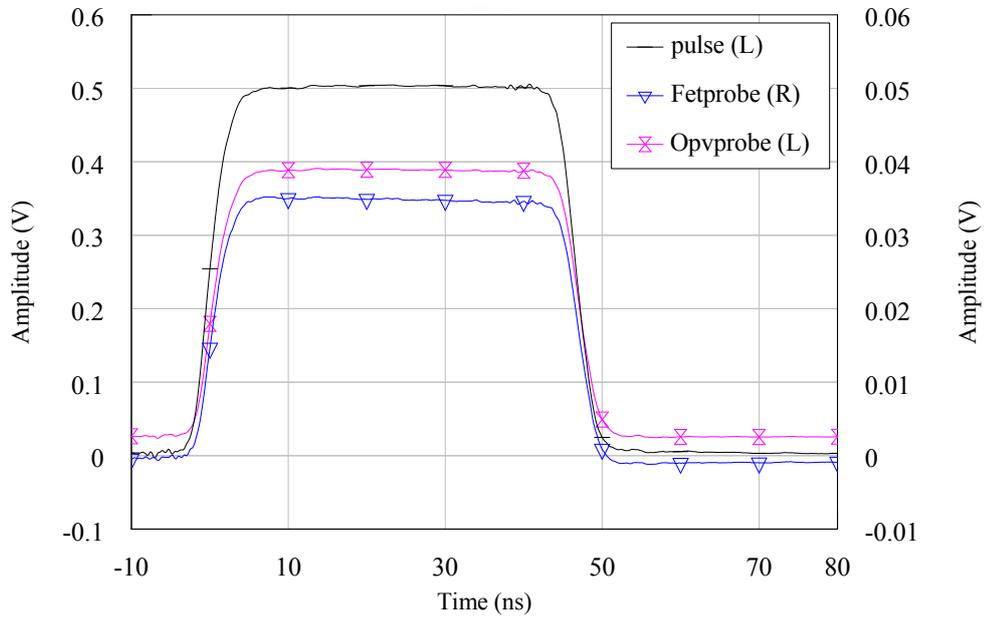
**Figure 3.9:** responses of both active probes to 500mV 50ns pulse
