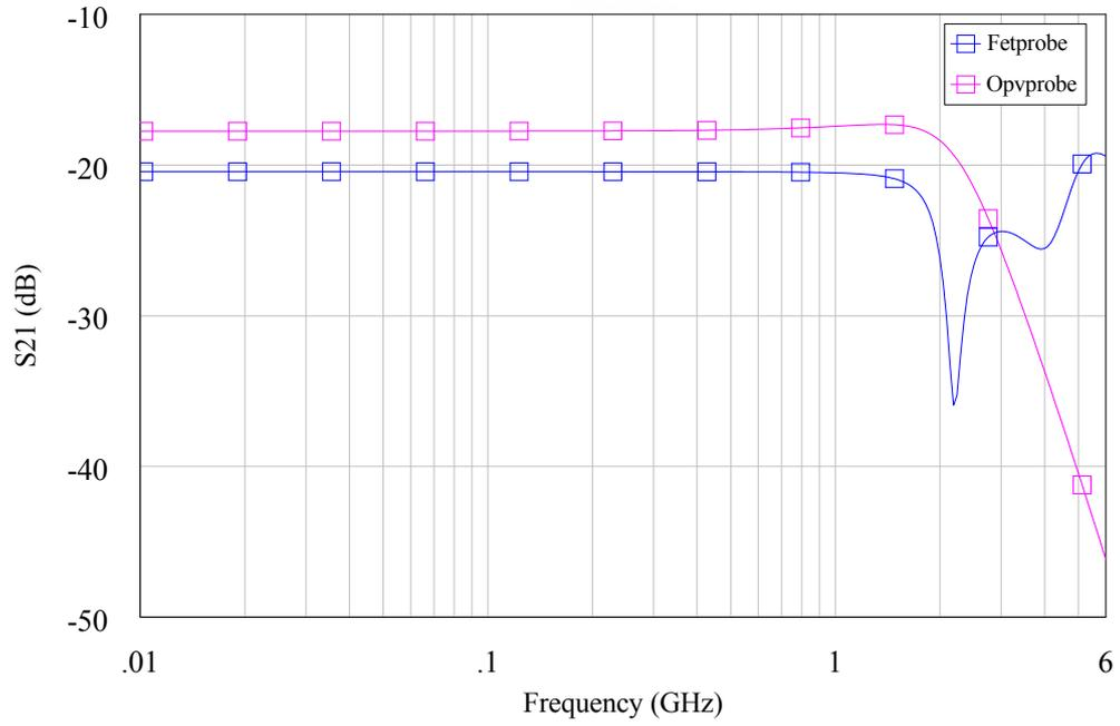
Figure 2.6: S21 of Fetprobe and Opvprobe
