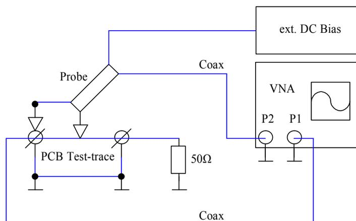
**Figure 3.1:** schematic of test trace
