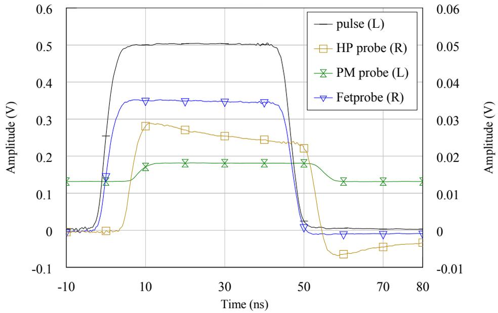
**Figure 3.20:** responses of both active probes to 500mV 50ns pulse
