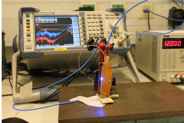
**Figure 3.4:** measurement setup for S-Parameters
