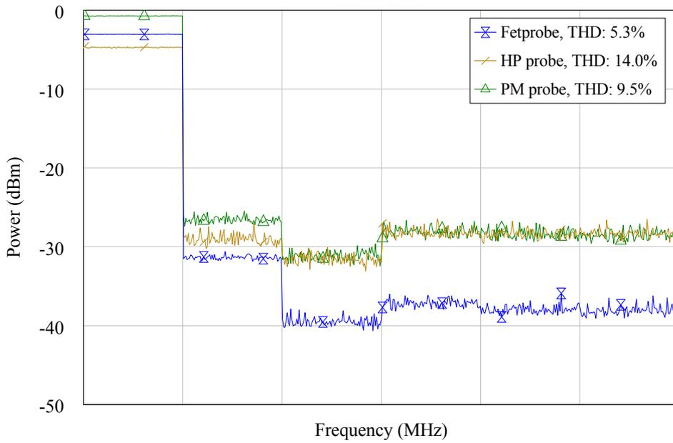
Figure 3.23: THD of Fetprobe and commercial probes (10 MHz@20 dBm)
