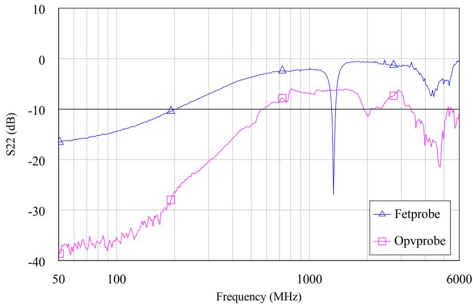
**Figure 3.7:** Output return loss of both active probes
