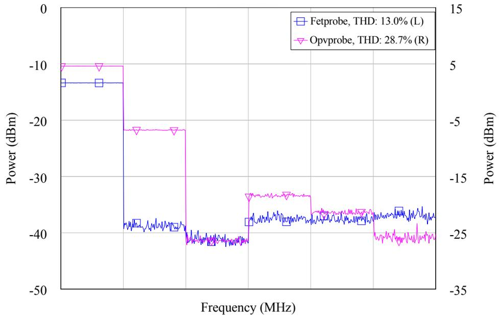
Figure 3.14: THD comparison of both active probes (100 MHz@10 dBm)
