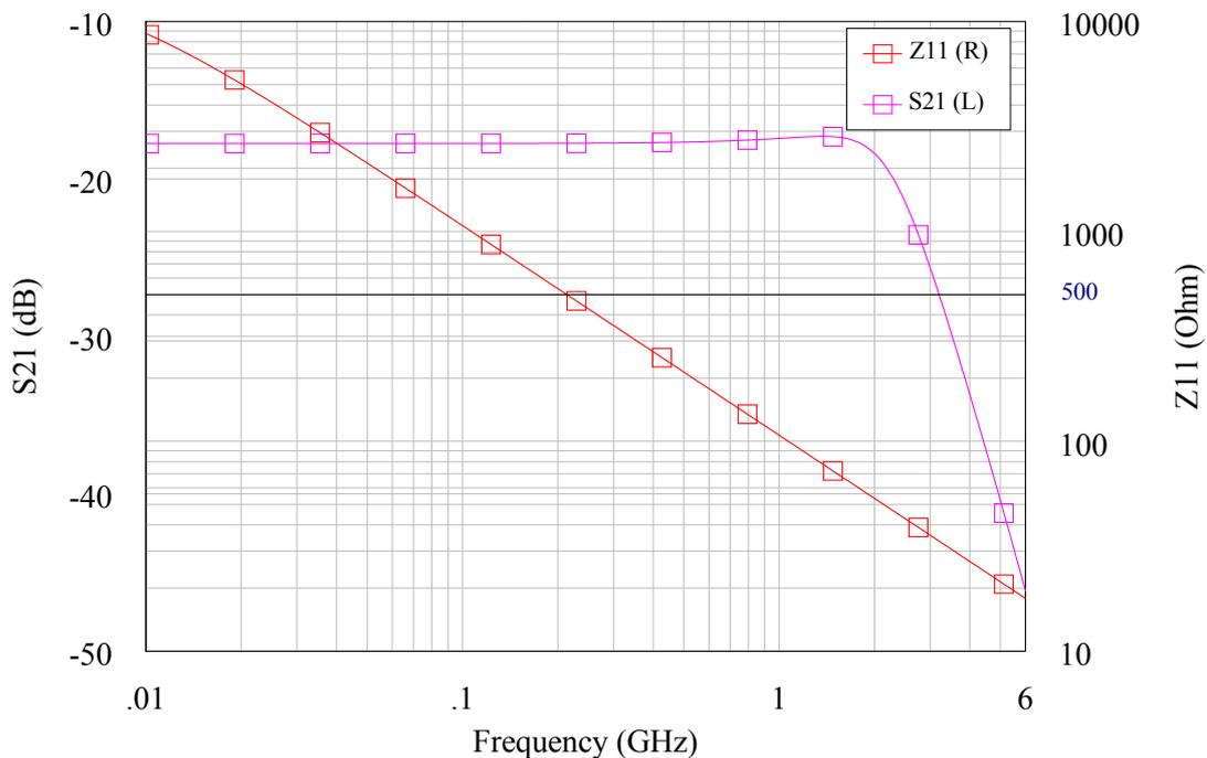
**Figure 2.8:** performance of the Opvprobe when simulating a  $500\ \Omega$  input resistor
