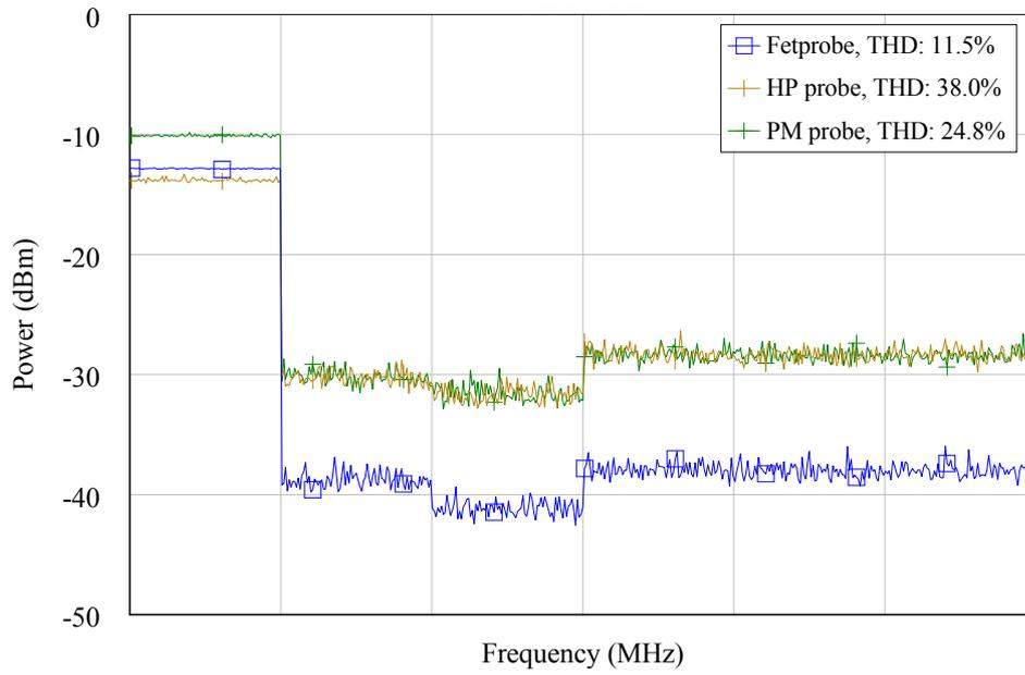
Figure 3.22: THD of Fetprobe and commercial probes (10 MHz@10 dBm)
