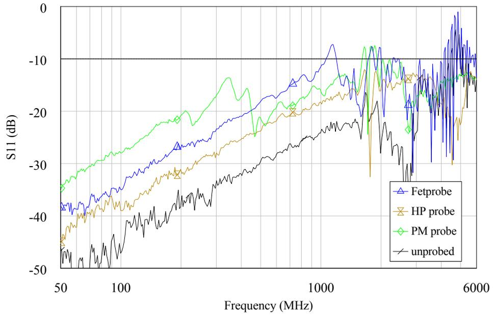
Figure 3.18:  $S_{11}$  of Fetprobe and commercial probes
