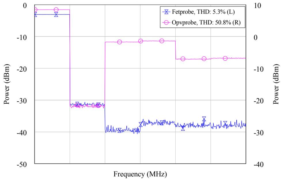
Figure 3.13: THD comparison of both active probes (10 MHz@20 dBm)
