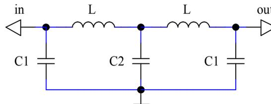
**Figure 2.4:** Fetprobe output filter
