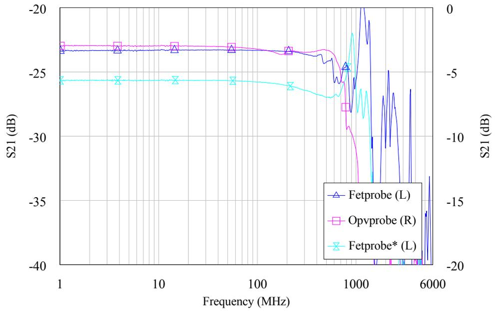
**Figure 3.5:** Transfer function of both active probes
