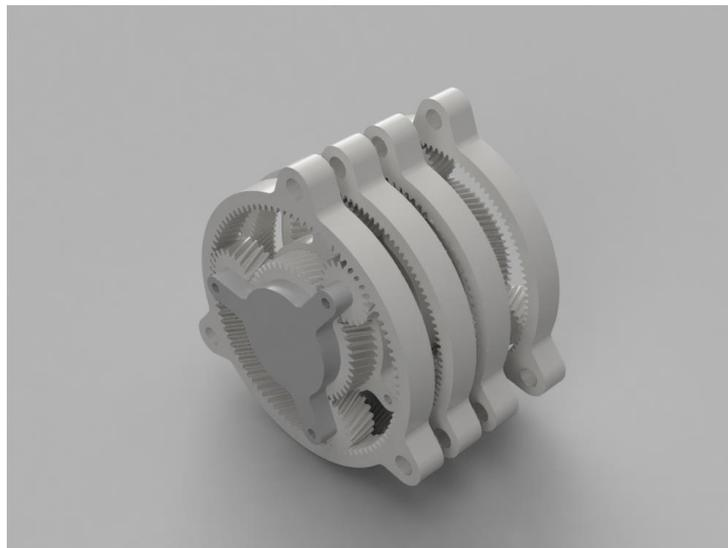
Figure 10: Final Planetary Gearbox CAD
