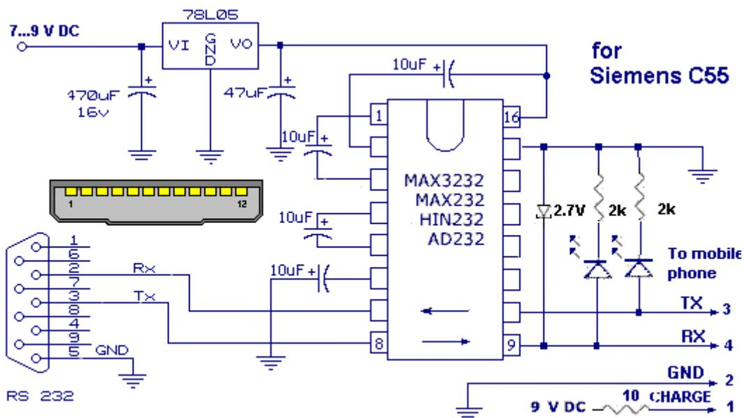
Siemens phone data connector I built first from a charger cable. It only has 2 pins and it takes some work to gluing in 2 more gold-plated contacts taken from a PC RAM memory connector. A much better solution is to buy headset and use the connector since it has all the 12 pins. Headset is usually cheaper than to buy just a new connector in your electronics shop.
