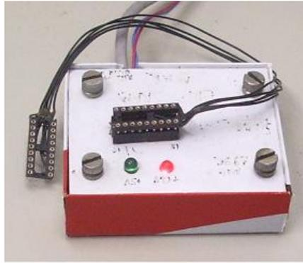
Notice a 5-wire in-circuit-programming adapter that saves time on removing the processor from sockets.
