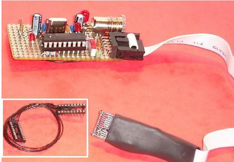
Note a 5-wire in circuit programming adapter works and greatly saves time on removing the processor from sockets.
