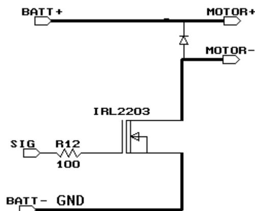
This circuit is used to control high current DC motors in radio-controlled electric model community. Several FETs can be put in parallel. They are
