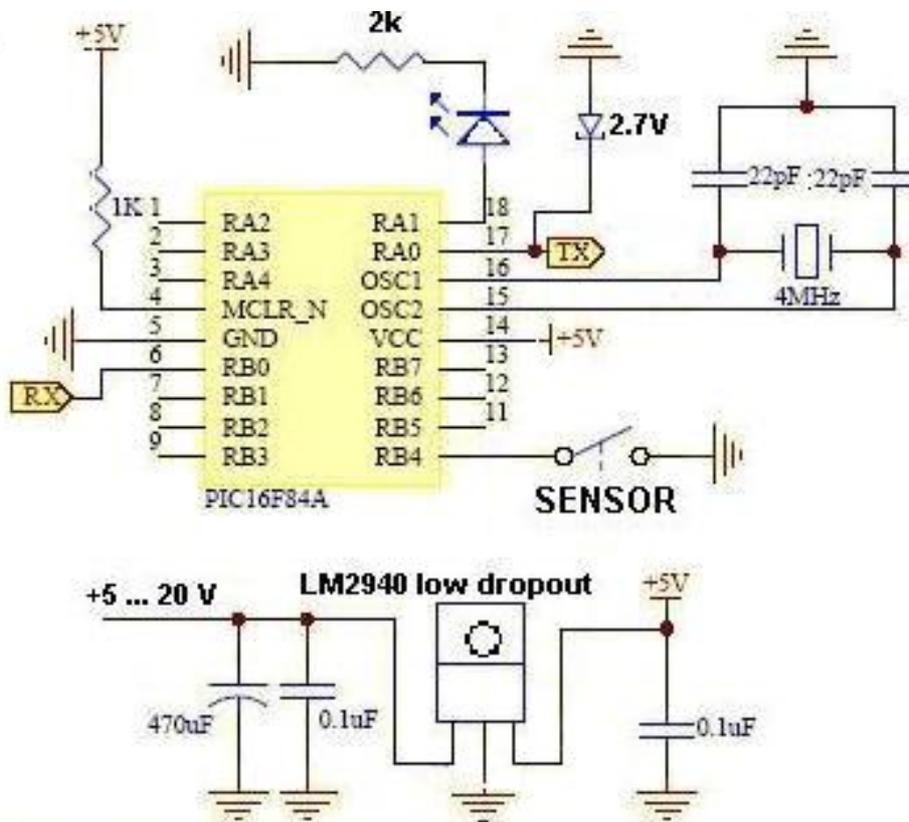
The circuit diagram is simple. The RX, TX and GND signals go to the phone via the cable that we made for the data cable board. There are many free pins that can be programmed for additional functions. It is assembled on a prototyping breadboard allowing to modify the schematics easily.
