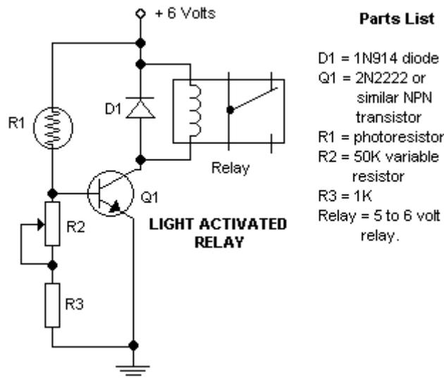
None of the parts of the light sensor are critical. Use potentiometer to adjust the level during light ON phase.
