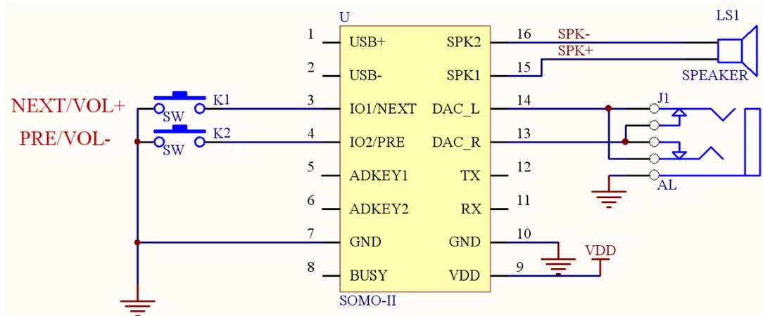
This is an example schematic showing the simplest connections to the SOMO-II for KEY MODE. Only 2 buttons are required. NEXT/VOL+ will start playing a track if currently stopped, and will raise the volume if the button is held down for > 1.2 seconds. PRE/VOL- will start playing a track if currently stopped also, and will lower the volume if the button is held down for > 1.2 seconds. See the table in Section 5.3 for more information.
