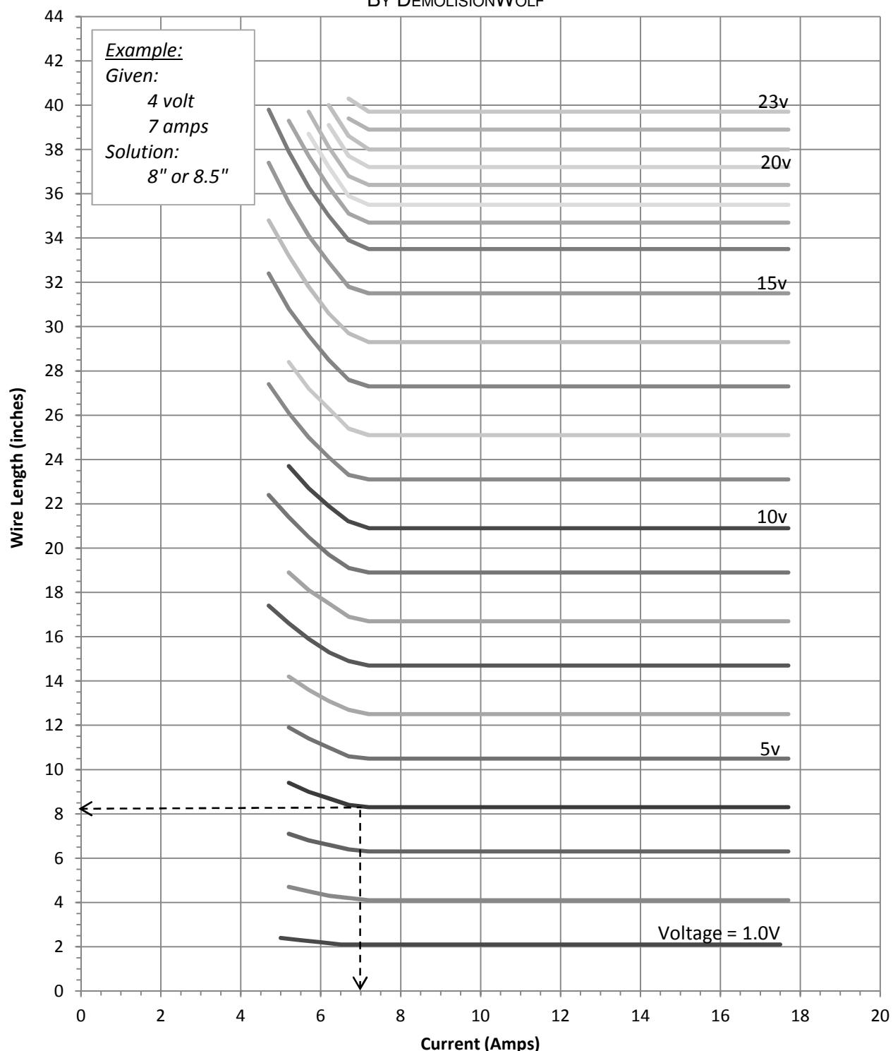
\* To increase temperature of wire during testing, decrease length by 0.5" increments.
