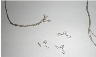
**Plate 1: Twisted Conductive Threads and Modified LEDs**
