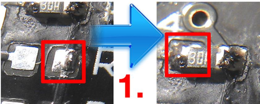
This type of SMD component is the easiest to solder: Apply a **very small amount** of **SOLDERING TIN** to **one** pad (1). If
