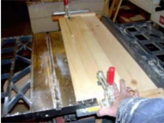
2 - A taper jig on the table saw, works best for the back slats and back supports E. A shop built sled is the quickest, easiest and safest taper jig. Use a scrap length of 6" (15.8 cm) wide plywood, longer than back slat I, and fasten clamps at each end. Extend the pattern lines to be cut, to the ends of the board using a straight edge. Line up the pencil marks with the edges of the sled and run it through the blade.
