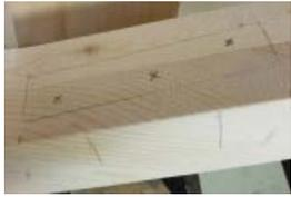
17 - Once the rockers are mated in the position you want, mark a pencil line around each front leg part D and the back ends of parts A and E. This will give you a marking to drill pilot holes for the screws in the correct locations.
