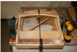
4 - Next attach the front slat C, with 2 screws on each side, to the front edges of parts A, flush with the bottom edges. This will give you a carcass to work with. Double check for square by measuring corner to corner, both ways. You can now remove the clamps and assembly square.
