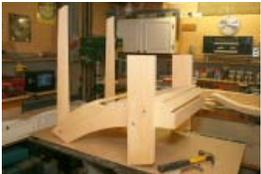
8 - Bolt on the back supports E, on the INSIDE of side panels A, being sure they are flush to the mated bottoms of the side panels parts A.
