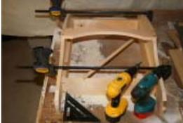
3 - Begin assembly by screwing the bottom back support part B, to the slot in each part A, the side panels. Use 2 screws on each side of part B using the hole locations provided on the templates. Be sure to drill pilot holes into parts A.
