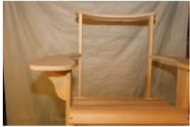
11 - Screw the arms G in place, as they rest on the front leg supports. Double check to be sure the arms are parallel to the ground. If not using pocket holes, put 2 screws through the arms into front legs D, and 1 into supports F. They should overhang the back edge of the front legs by 1/4" (6mm), leaving about 19 1/2" (49.6cm) between the arms. Put 2 screws in from the inside of parts E, into the notch at the back of the arm. Check to be sure the arms are parallel to the work surface.
