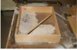
1 -If you are building a few chairs, you may want to begin assembly by using scrap boards to make an assembly box to clamp parts A, the side panels, to make it easier to attach part B & C, so the frame is square. Mine is 4" (10.2 cm) high by 24" (61 cm) long....the important dimension is the width of 19 1/2" (49.6 cm). When you clamp parts A to each side, it will equal the 21" (53.4 cm) width of parts B & C as well as all the seat slats.
