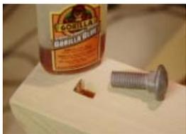
23 - If the front legs are slightly off square like mine was, and the legs fit flush, you can add weight to the underside of the rockers as a counter balance. I cut two 3" x 1/2" (4.8cm x 1.2cm) galvanized carriage bolts to 1 1/2" (3.8cm) long, and glued them in holes at the back ends of the rockers. The chairs balanced perfectly, and the curved bolt heads act as a safety stop, if the chair is rocked backwards too far.
