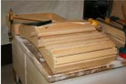
6 - The rest of the seat slats can now be assembled and attached using one screw on each side. Evenly space all slats M using 2 strips of 1/8" (3 mm) hardboard as spacers, or one strip of 1/4" (6mm). Add part N, the back seat slat. The spacers should evenly space all slats back to part B. Be sure to double check the squareness when screwing in each slat.
