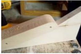
18 - Use a tapered scrap cut off, as a support when drilling the pilot holes completely through the rockers. Be careful not to drill on an angle, or the screws may penetrate the edges of the leg parts. An easy reference is pencil lines on the rocker that align with the legs. You may need to extend the drill bit as far as possible, so it will penetrate the bottom of the rocker.
