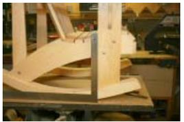
16 - Once you are comfortable that both rockers are identical, place the chair on the rockers, set out 5" (12.7cm) from the front legs parts D. They should be close to the ends of the arms. Using a square adjust the positioning on the rockers to get the legs perpendicular. You may need to sand the under side of the front legs and side panels to get a perfect fit. You can center the legs straight on the rockers, or angle the rockers in at the back like I have.
