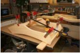
2 -This is an alternative option using standard assembly squares and clamps. Clamp parts A to your assembly squares, being sure that the fronts are even and square. Raise the parts at the front with a board, to ease in screwing on part C.
