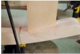
20 - Line up the rockers with the pencil marks at both ends and clamp the rockers firmly to the legs, with the other end of the clamp on the seat slats.
