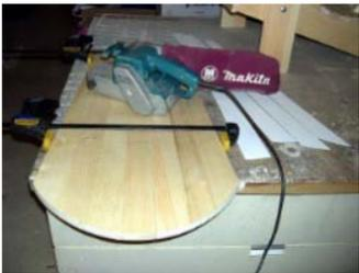
3 - For all back slats, cut to the rough dimensions of part I, the longest slat. Then trace on template I, and taper the one side for all parts I, J, K & L. The templates for J, K & L can be traced onto the tapered stock, so all parts are the same width at the bottom. Only one template of each is necessary. Just flip each over for the opposite direction of the curve. When you have cut & planed or sanded all slats, assemble & clamp as shown, so you can sand the curve smooth and even.
