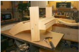
7 - Next, bolt on the front legs D, on the OUTSIDE of parts A. Use washers on the insides and hand tighten for now, to allow some movement when attaching the rockers. Use the 2 1/2" (6.35cm) bolts.
