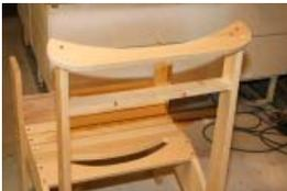
9 - Screw on the upper back support H, centered on the tops of parts E, flush at the front with supports E. Use an 18" (45.7 cm) scrap spacer, as shown, to be sure the back supports are parallel to each other.
