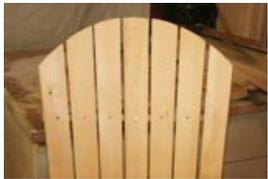
13 - If you are using plugs to hide the screws, be sure to add them NOW, to the bottom of the back slats, and sand smooth. Then you can re-install part N.
