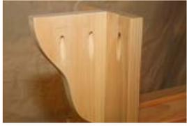
10 - With two screws, attach the arm supports F, centered flush with the top of the front legs D. If you have a pocket screw kit, you may want to follow the images below and the pocket screw kit instructions, to attach the arms from the underside, instead of from the top of the arms. Use shorter screws, practice on scraps, to be sure you don't screw through the top of the arms.
