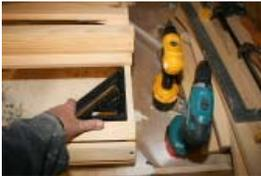
5 - Using a square, screw one of the seats slats M above part C, so it is even with the upper edges of the pattern on parts A. This will leave a 3/16" (5 mm) space. Do the same for the next slat. All slats are 21" x 1 3/4" x 3/4" (53.4 cm x 4.5 cm x 1.9 cm), and templates are not required.
