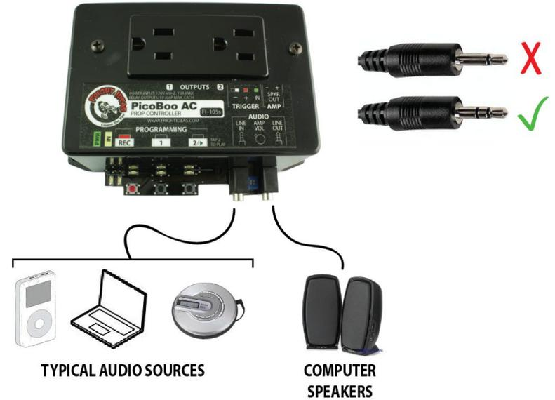
Once the above is connected, press play on the audio source and you should be able to hear the sound faintly through the connected speaker. DO NOT turn up the source volume so your speakers are really loud! Use this sound only as a guide so you know when to start and stop recording. Once the sound is recorded and the PicoBoo plays it back, it will be much louder than it is now.
