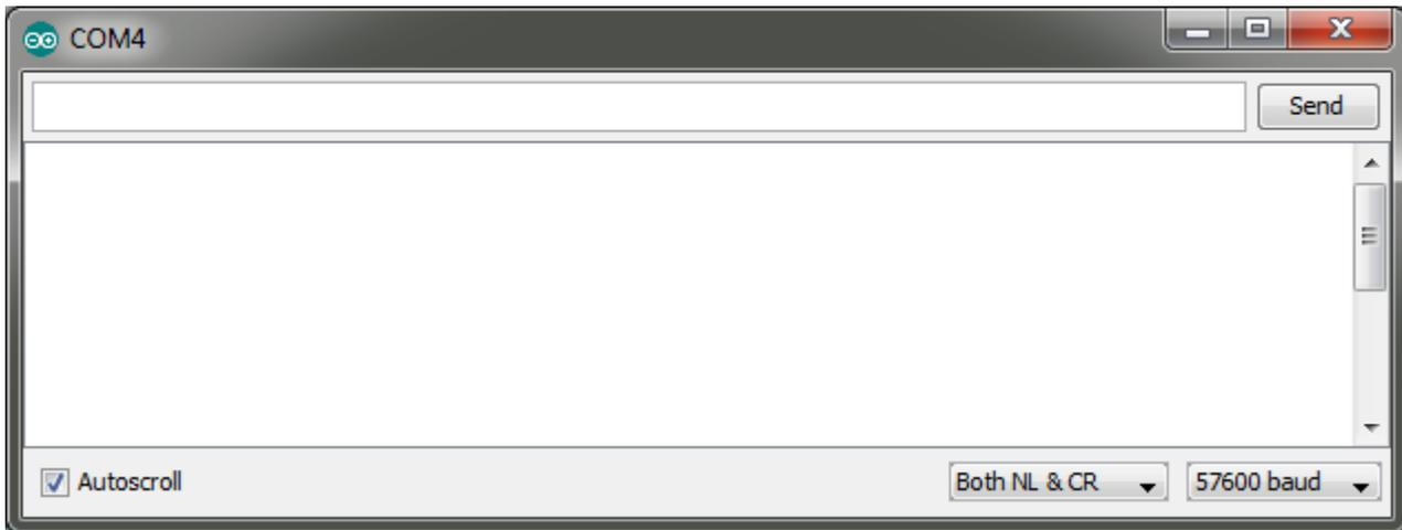
Before trying out some of the available commands go ahead and check that the controller is currently not applying any force on the motor. Try to move the shaft of the motor and notice that it rotates freely. Now type 1 on the serial monitor and press enter.
