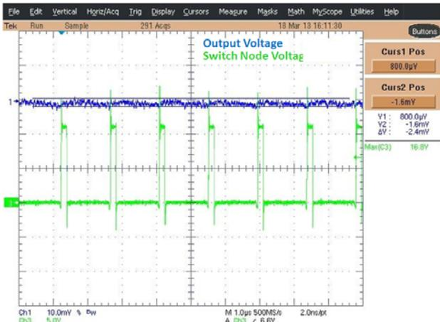
Figure 7. Ripple Voltage for 3200 µF Capacitance
