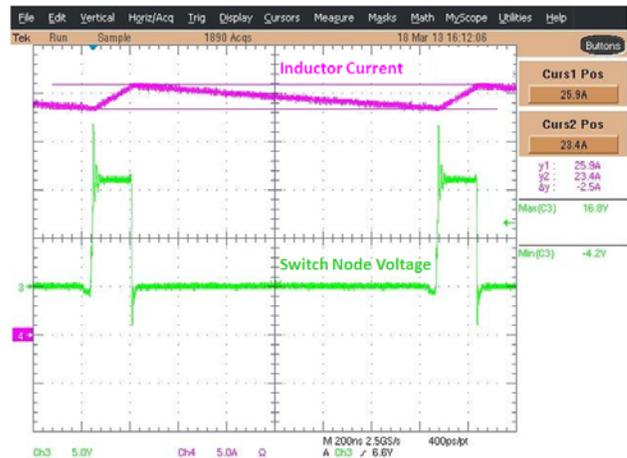
**Figure 5. Ripple Current for 0.82 μH Inductor**
