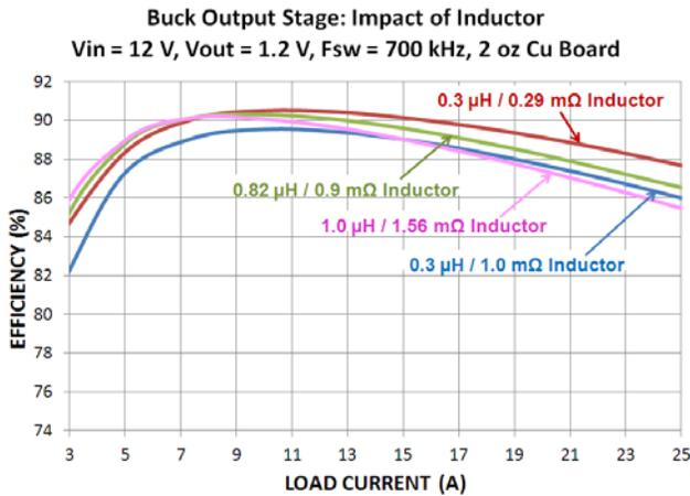
Figure 10. Effect of Inductance on Efficiency
