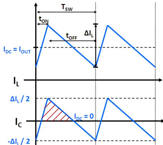
Figure 3. Inductor and Capacitor Current
