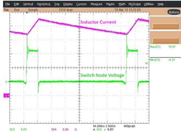
**Figure 4. Ripple Current for 0.3 μH Inductor**
