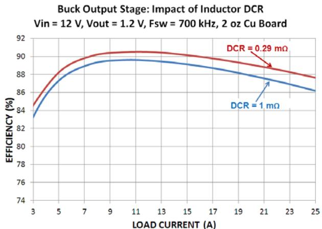
Figure 9. Effect of Inductor DCR on Efficiency
