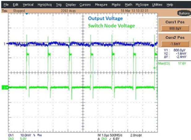
Figure 6. Ripple Voltage for 1600 µF Capacitance
