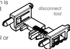
**NOTE:** To remove a sealing cap, you must use the Enphase disconnect tool or a #3 Phillips screwdriver.
