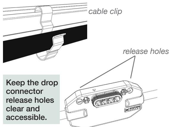
Keep the drop connector release holes clear and accessible.
