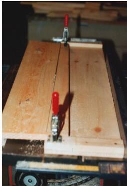
For the back slats, parts I, J, K & L, unscrew the bottom clamp board, and line it up with the bottom end of the sled as shown. This will give you the extra length necessary. You can also get fancy, and insert aluminum channels into the sled base, to allow you to use screw clamps to slide the bottom toggle board to whatever position you need.
