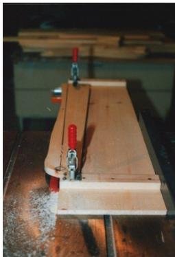
Rough cut out traced part E from the original board, and place it on the sled, lining up the side to be cut with the left edge of the sled. You may want to extend the line of the pattern to the ends of the rough sized board, to allow for easier alignment. You can also use a T-square to line up the traced pattern to the edge of the sled.
